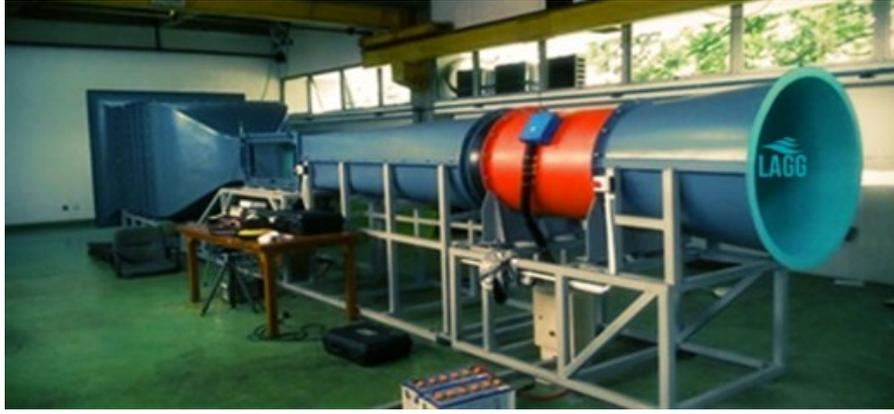
Figure 2. ESWT wind tunnel
